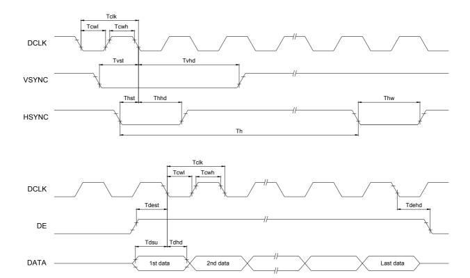
3.5 Input Signals Timing Characteristics
