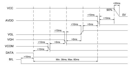
Power off sequence:  $B/L \rightarrow DATA \rightarrow VCOM \rightarrow VGH \rightarrow VGL \rightarrow AVDD \rightarrow VCC$
