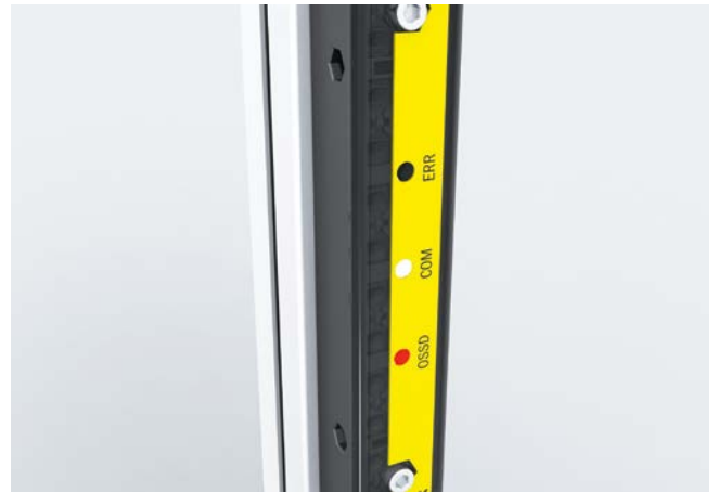
2. When the mounting surfaces are properly aligned, the white COM LED lights up continuously.
