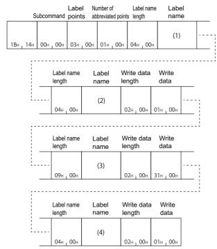
In the figure (1) to (4), set the value of "Binary code" indicated in the table of "Value of code corresponding to character" of each label name.
