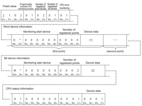
In the figure (1) and (2), set the value of "ASCII Code" in the table of "Device data" of each response data. The order of device data differ depending on the setting of "Word/byte units designation" in Engineering tool.
