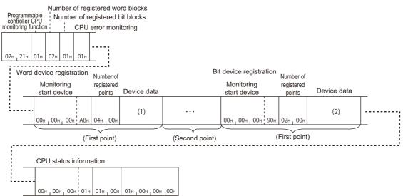
In the figure (1) and (2), set the value to "Binary code" in the tables of "Device data" of each response data. The order of device data differ depending on the setting of "Word/byte units designation" in Engineering tool.
