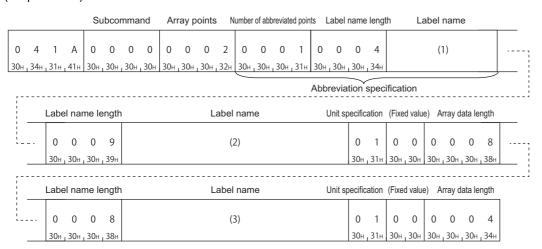
In the figure (1) to (3), set the value of "ASCII code" indicated in the table of "Value of code corresponds to character" of each label.
