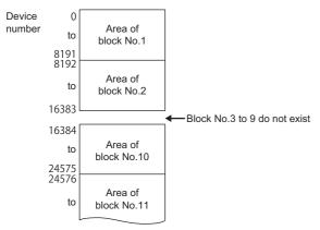
The following table shows the range of device numbers to be specified when using AnA/AnUCPU common commands for 28 blocks per each block.
