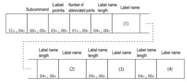
In the figure (1) to (4), set the value of "Binary code" indicated in the table of "Value of code corresponding to character" of each label name.
