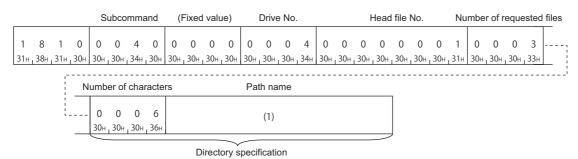
In the figure (1), set the value of "ASCII code" in the table of "Value of code corresponds to character" in "Path name". (Response data)
