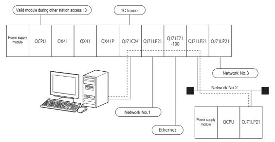
When accessing in accordance with the setting of "Valid Module During Other Station Access" using a frame with the network No. set is desired, specify 'FEH' (254) to the network No.
