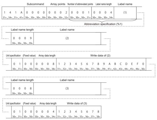
In the figure (1) to (3), set the value of "ASCII code" indicated in the table of "Value of code corresponding to character" of each label name.
