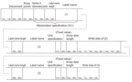
In the figure (1) to (3), set the value of "Binary code" indicated in the table of "Value of code corresponding to character" of each label name.
