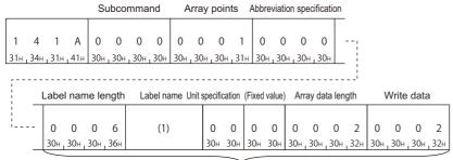
Array specification (Array one point)
